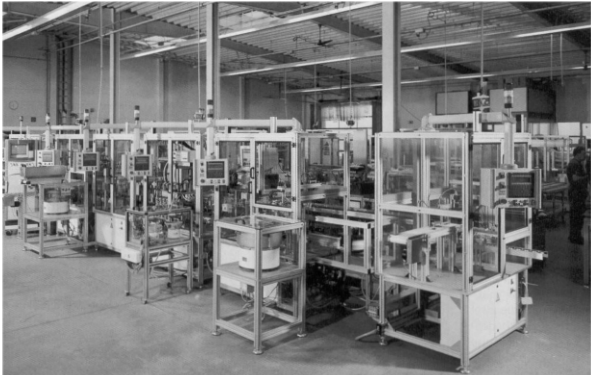
Figure 28: Mounting and checking of car Xenon headlight
