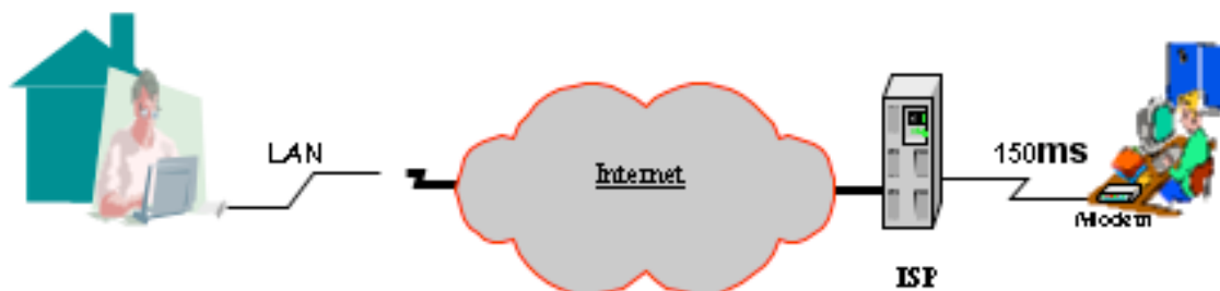
Figure 3. The LAN - Internet - modem environment in Stage 2 of the evaluation of NetMeeting
