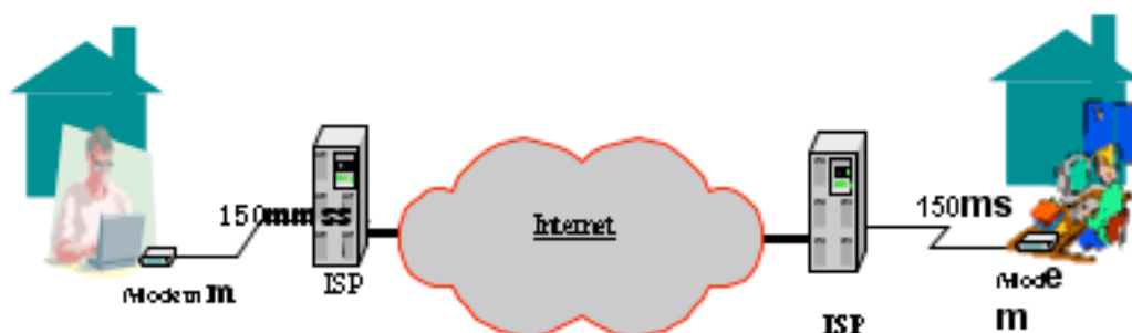
Figure 2. The modem - Internet - modem environment in Stage 2 of the evaluation of NetMeeting
