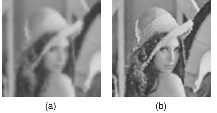
Figure 3: Grayscale lenna test image reconstruction with 10% of samples: (a) using f = 1 , (b) f = 1/8
