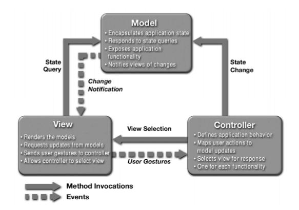
**Figure 2:** The Model-View-Controller (MVC) Design Pattern (Source: Sun Microsystems. <a href="http://java.sun.com/blueprints/patterns/MVC-detailed.html">http://java.sun.com/blueprints/patterns/MVC-detailed.html</a>)
