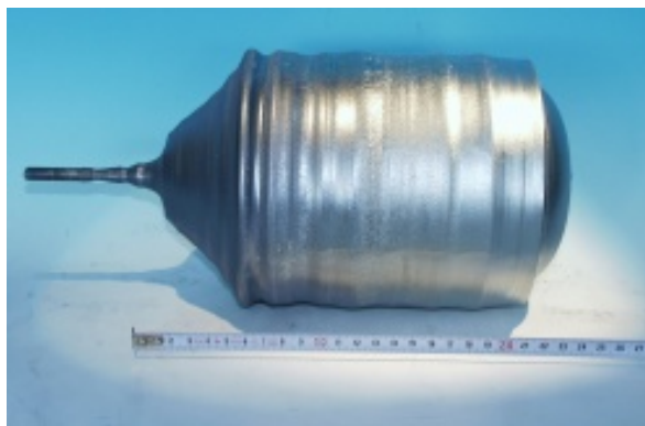
Figure #14: Freiberger GaAs crystal (source: http://www.fcm-germany.com/ ).
